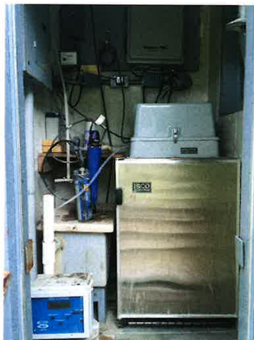
Figure 2. Inside of the shelter for the sampling station showing the flow through tank on the left and refrigerated sampler on the right.
